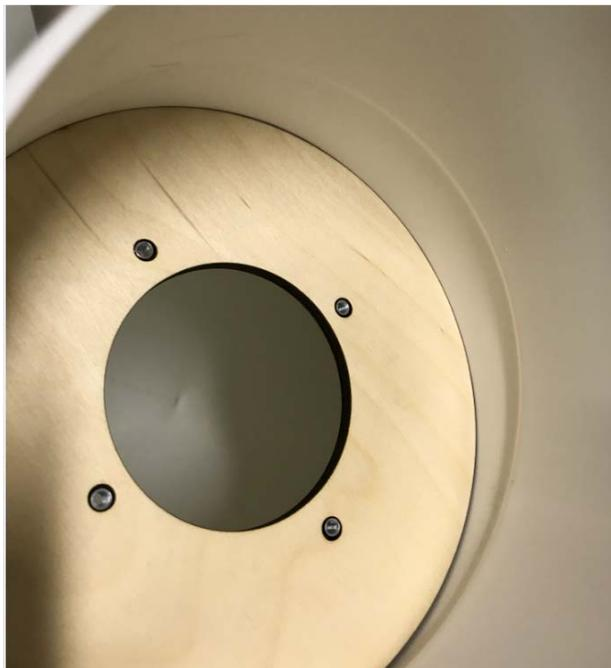
4. Pull the ring toward the cone shoulder until the ring is flush. When satisfied with the fit epoxy the ring into place bonding the ring to the cone. Forward and aft ends are OK to do currently. Don't get any epoxy in the T nuts!!!
