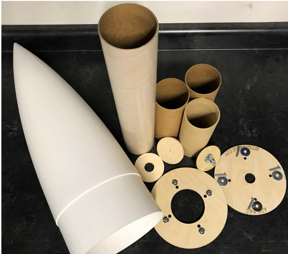
1. Use 80 grit sandpaper to score the inside of the cone. This will help the epoxy adhere to the plastic. Wash the inside of the cone with dish soap and warm water after sanding is complete.
