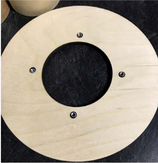
3. Squeeze cone a few millimeters and insert ring into forward end.
