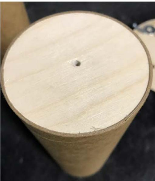
8. Choose a good material to make your nose weight. We typically use zinc pellets. Always simulate your flight with preferred motor to determine the amount of ballast to use. Additional couplers and materials can be purchased to make alternate weight variations for the nose cone. Smaller motors need less weight, larger motors need more weight. **ALWAYS SIMULATE YOUR FLIGHT!**
